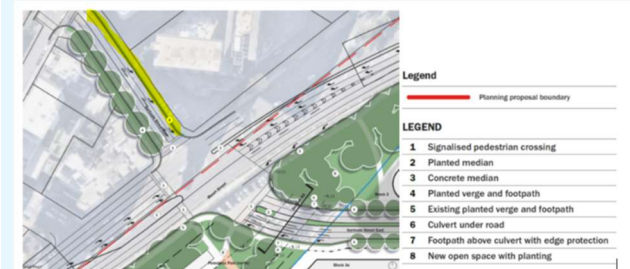
Figure 205 – Indicative Marsh Street and Gertrude Street intersection upgrade and extension
